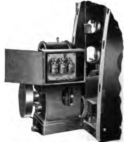
Fig. 3. Enclosed Switchboard for Motor-Driven Planer.
